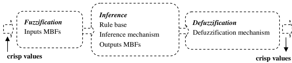
Diagram 5. Fuzzy logic system blocks
